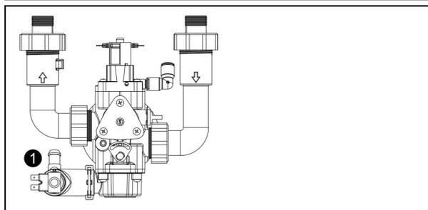
1. Install the drain adaptor with air gap to the sewerage system.
