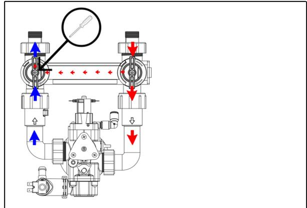
1. Adjust the residual hardness of the water that leaves the softener, by means of the adjusting screw, incorporated in the 'outlet' valve of the factory bypass:
