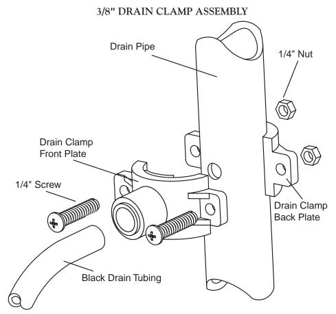
to Hose Barbs. Route the tubing to the Drain Clamp and trim to length.
