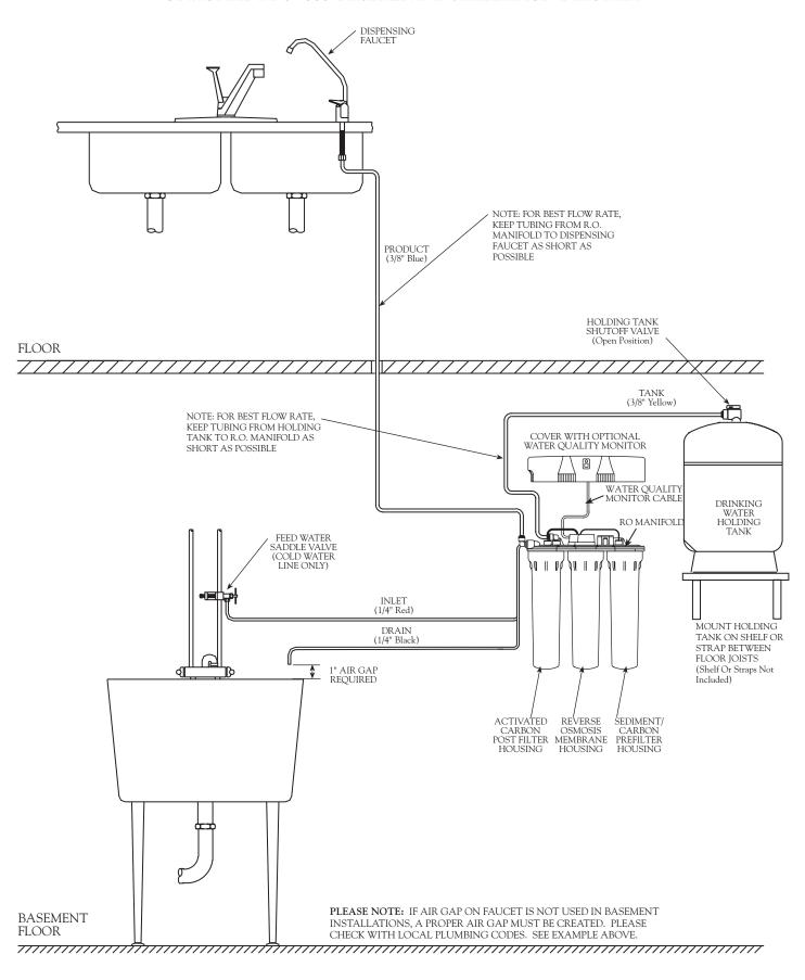
system cover for instant monitoring at the touch of a button. The monitor compares the level of the total dissolved solids in the incoming (feed) water versus the product water and calculates the percent rejection. The monitor is preset to indicate a level of 75% rejection. NSF/ANSI Standard 58 requires a 75% total dissolved solids rejection to pass the requirement of the standard.
