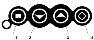
1. **SET**. Used to accept a setting to be stored in memory or to allow a setting change.
